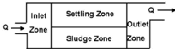
Figure 9.1: The four functional zones of a continuous flow settling basin
