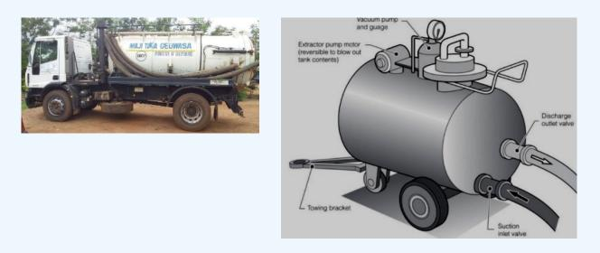
Figure 4-4: Typical Vacuum Tankers (Left); Typical Portable Vacuum tank (Right)
