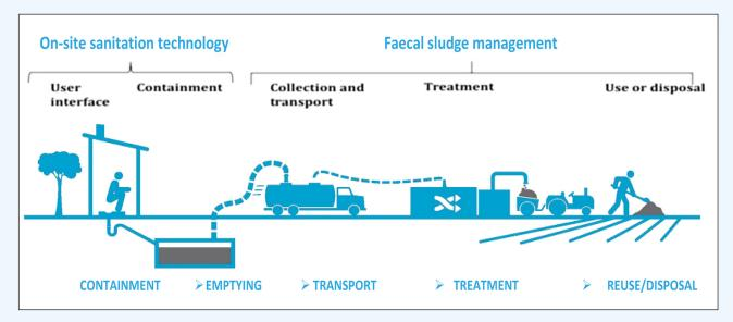
Figure 1- 1 Segments of sanitation Service Chain (Adapted from Design, Construction, Operation, Maintenance Manual, MoW 2020)
