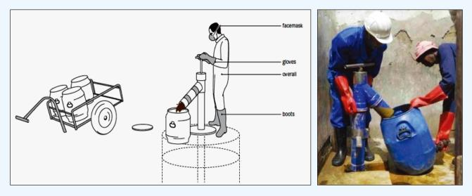
Figure 4- 1 Gulper Technology (Left); Emptying using the Gulper (right) (Adapted FSM Guide for Dar es Salaam, BORDA 2019).
