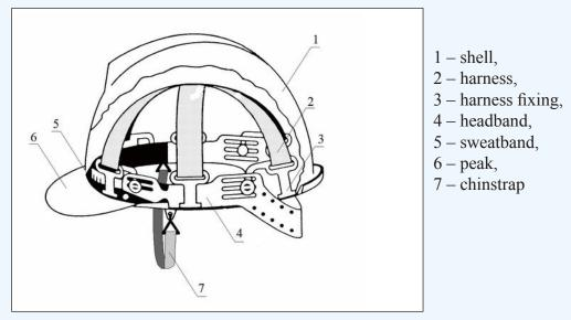
Figure 2: Construction of an industrial safety helmet.
